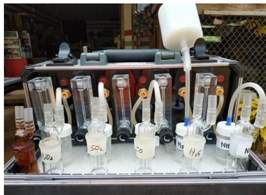
Gambar 1. Gas Sampler Impinger
